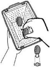
**6.** Insert Print Lamps into the Lamp Housing by inserting and twisting until they are locked in place. You will note the lamps only twist in one direction.
