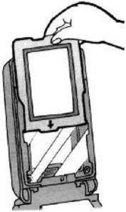
1. Insert the inked up Print Master into the PG-5 machine
