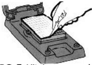
**IMPORTANT:** Place a blank piece of card onto the Pad Table, which is now adhesive, to avoid the Stage Glass adhering to the Pad Table once the Lid is lowered.
