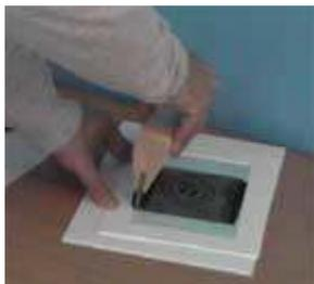
When complete, raise the squeegee angle back to vertical to 'pick up' the ink and remove from the squeegee from the screen
